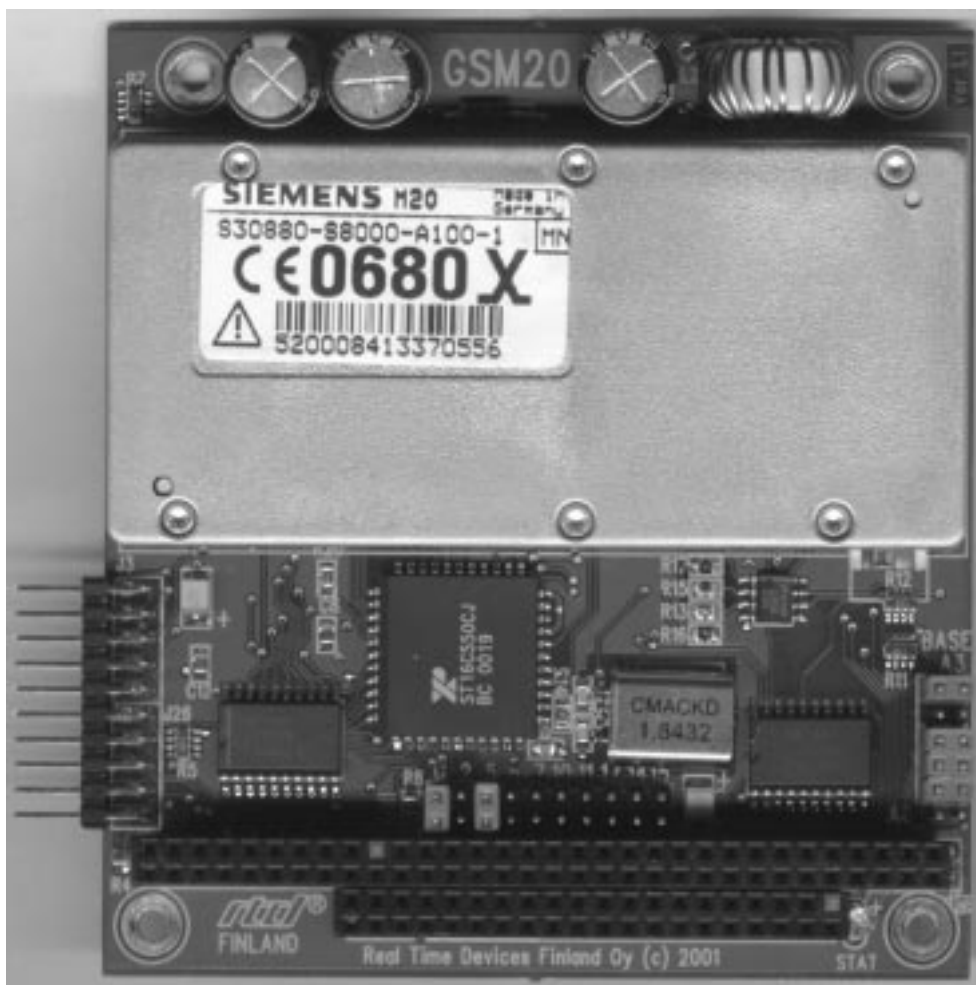
Fig. 2-1 GSM20 Board layout showing jumper locations
